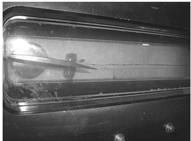
FIG. 2. Photograph of the hydrofoil in the water tunnel test section with developed tip-vortex cavitation with U_\infty = 10 m/s, and \sigma_\infty = 1.4 . Flow is from left to right.
